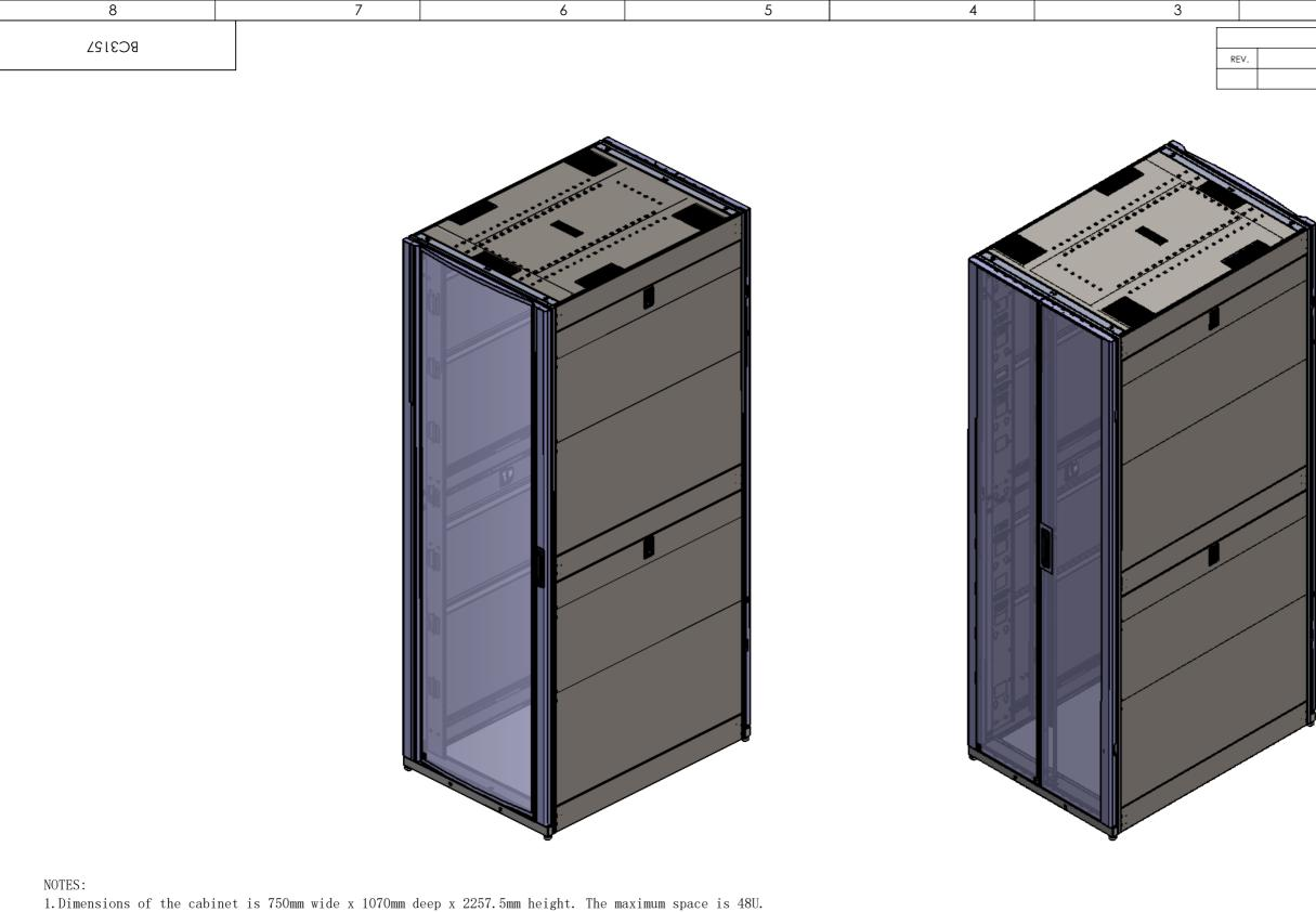
1.Dimensions of the cabinet is 750mm wide x 1070mm deep x 2257.5mm height. The maximum space is 48U. Surface is with RAL9005 black powder coated, with metallic luster.
